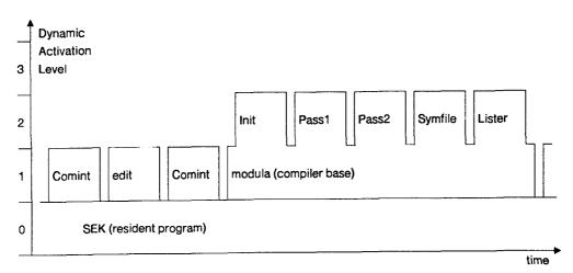
The figure illustrates, how programs may be activated. At a certain moment, the *dynamic activation level* or simply the *level* identifies an active program in the stack.
