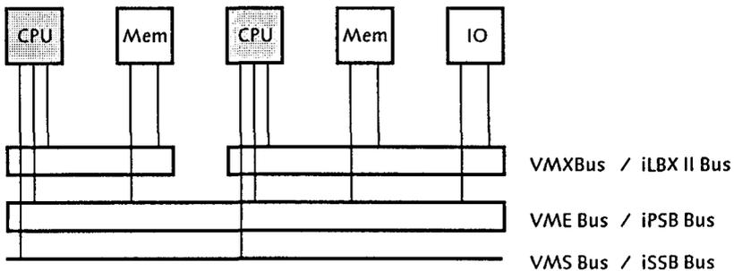
**Figure 4.18** VMEbus and Multibus II bus architecture.
