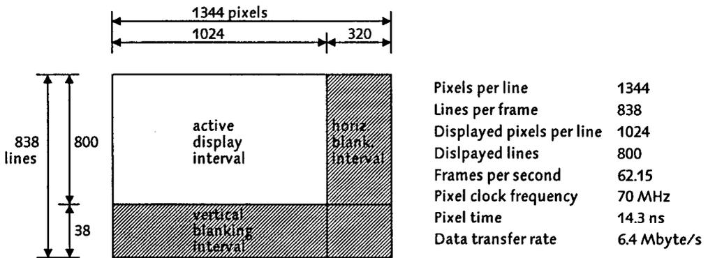
**Figure 2.12** The display parameters of the high-resolution CRT-monitor.
