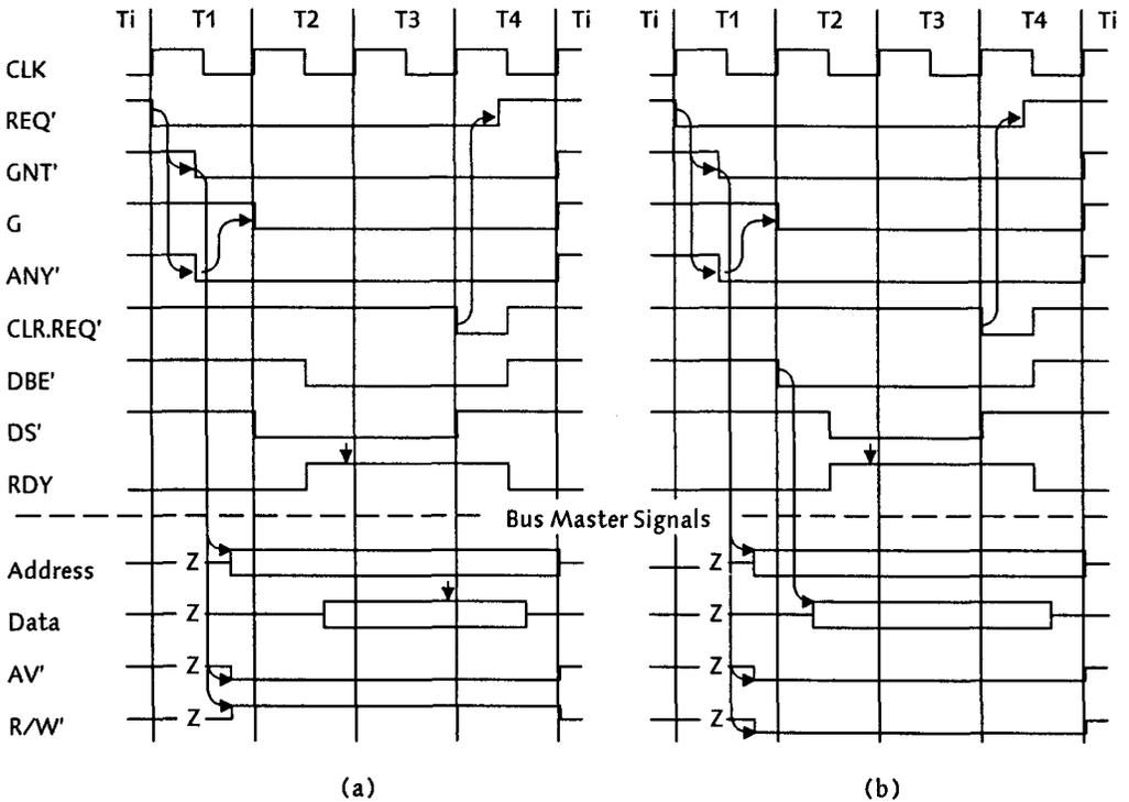
**Figure 2.5** Read (a) and write cycle timing (b).
