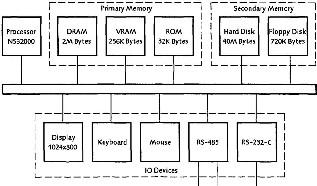
Figure 2.1 Hardware structure of the Ceres computer.
