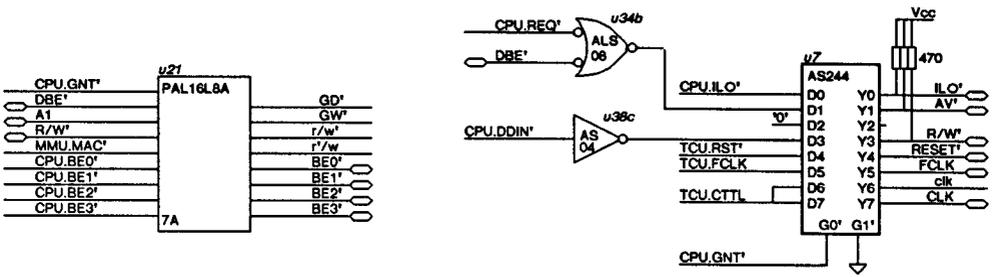
Termination resistors (270/560) are provided for TCU.FCLK, TCU.CTTL, FCLK, CLK and clk.
