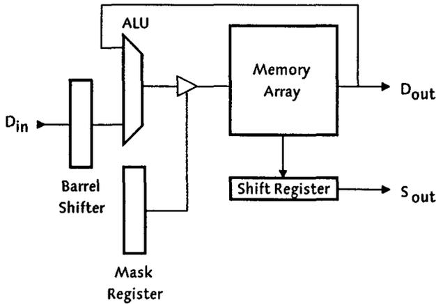
**Figure 3.8** Frame buffer with hardware assistance for RasterOp.
