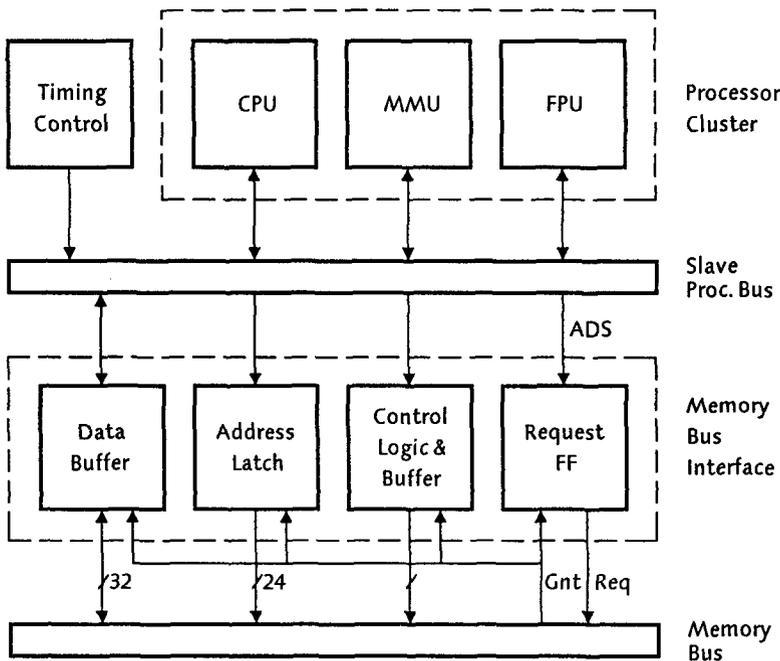
**Figure 2.2** The processor and its memory bus interface.
