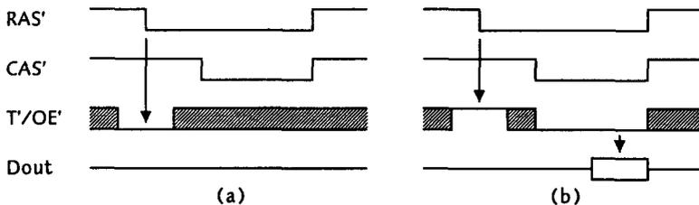
**Figure 2.15** VRAM shift register transfer (a) and random access operation (b).
