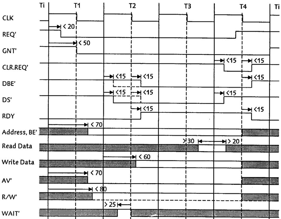
Figure 2.17 Timing specifications of a basic memory cycle.
