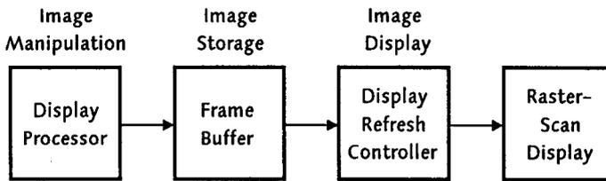
**Figure 3.1** Structure of a raster graphics system.
