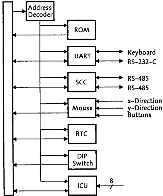
**Figure 2.7** Boot ROM and standard IO devices.
