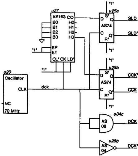
Termination resistors (270/560) are provided for dck, DCK, DCK', SLD, SLD'.
