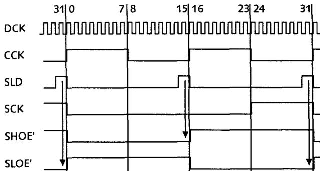
**Figure 2.14** Clocking signals of the display refresh controller.
