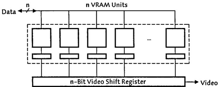
**Figure 3.6** Frame buffer organization based on VRAMs.
