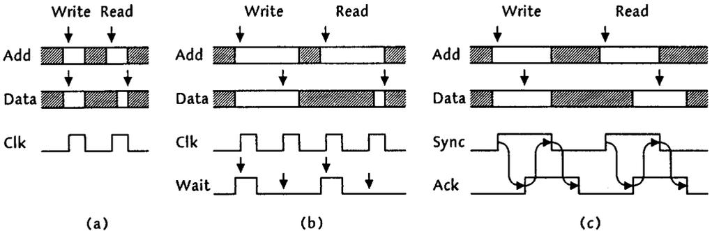
**Figure 4.8** Synchronous (a), semisynchronous (b), and asynchronous transmission (c).
